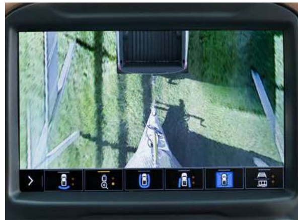
Rear Top-Down View Shows the clearance between the truck bed and nearby objects.
