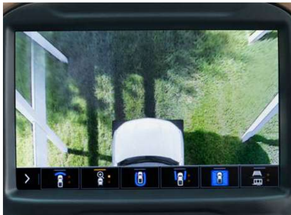
Front Top-Down View Provides a top-down view of the hood, bumper and front tires for tight maneuvers in parking lots or along curbs.
